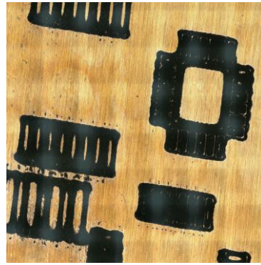
Area 1 - 0.2 mm diameter tool 2 passes
