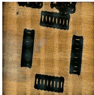
Area 5 - 0.2 mm diameter tool 2 passes
