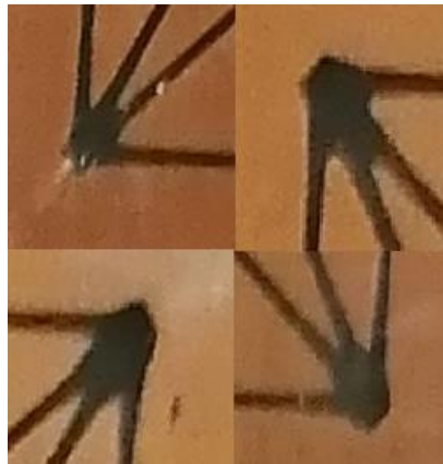
Figure 6.14 – Undesired dot pattern at the corners due to a long laser exposure
