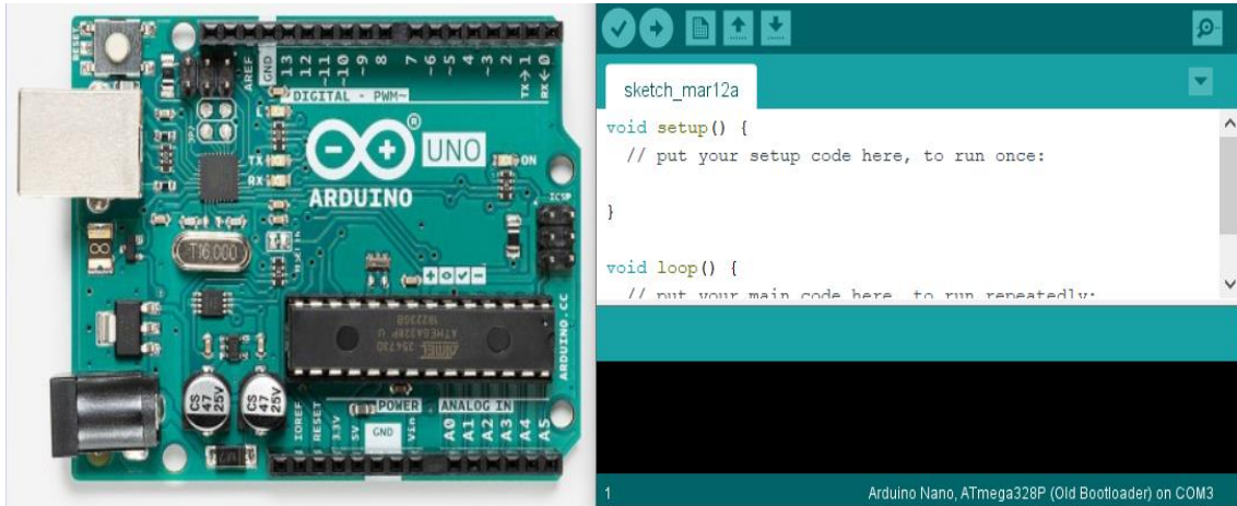
Figure 3.7 – Arduino hardware “Arduino Uno Rev3” (at the left) and Arduino IDE (at the right) (Source: Arduino’s official website (2021))
