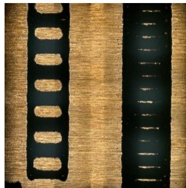
Area 6 - 0.2 mm diameter tool 2 passes
