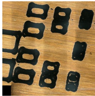
Area 4 - 0.2 mm diameter tool 2 passes
