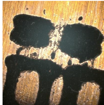
Area 3 - 0.2 mm diameter tool 2 passes
