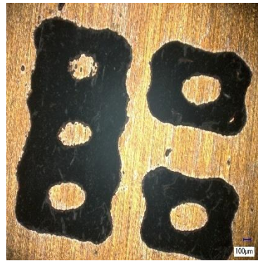
Area 2 - 0.2 mm diameter tool 2 passes
