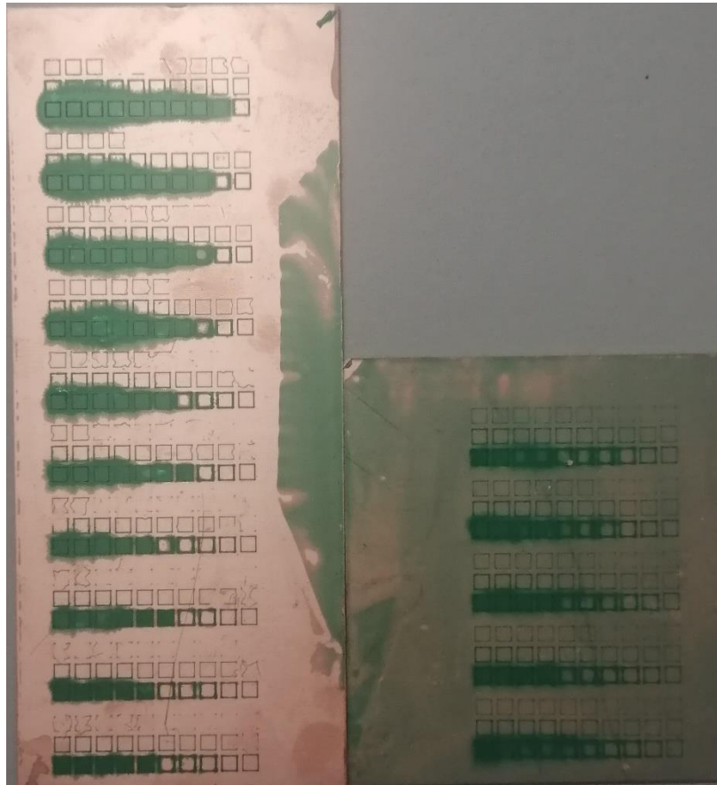
Figure 6.50 - DFSM solder mask printed pattern after development
