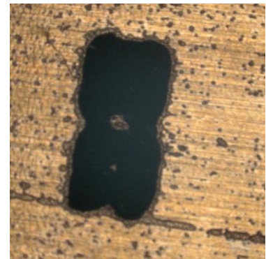
Area 4 - 0.1 mm diameter tool 2 passes
